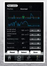
The customer can make the adjustments he wants to the regulation of the vertical acceleration (up-and-down movement), horizontal acceleration (transverse acceleration to the left and right) and longitudinal acceleration (accelerating and braking) through his iPhone.
